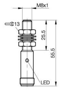
Inductive Sensors BES 516-377-E5-C-S 4 M8x1 x 55.5 normally-closed Sn=1,5mm shielded
